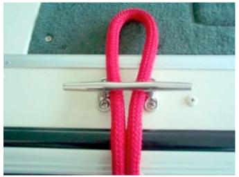
Next, bring each side of the loop over the cleats shank. This will provide a secure tie up to the boat cleat.
