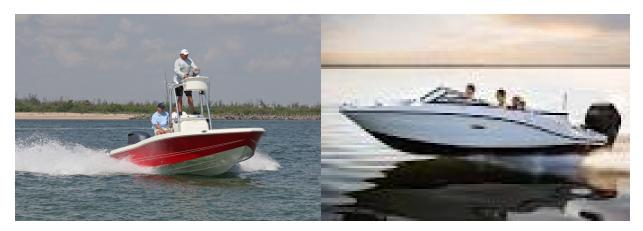
The photos illustrate the proper planning position. Notice the bow is up and the water line begins at about where the bow v of the hull stops and then goes straight.
